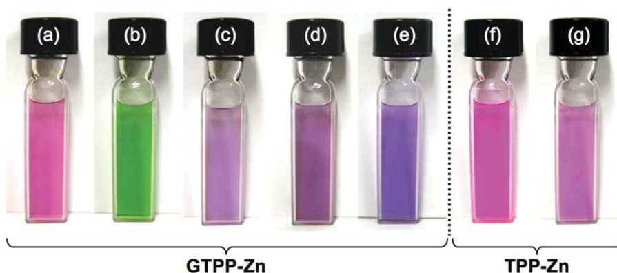
Fig. 2 Library of colour changes of the porphyrin derivatives (0.5 mM) in cyclohexane at 20 °C. (a) GTPP-Zn , (b) GTPP-Zn with pyridine (10 equiv.), (c) GTPP-Zn with pyridine (2000 equiv.), (d) GTPP-Zn in chloroform, (e) GTPP-Zn with pyridine (10 equiv.) in chloroform, (f) TPP-Zn , and (g) TPP-Zn with pyridine (10 equiv.).
